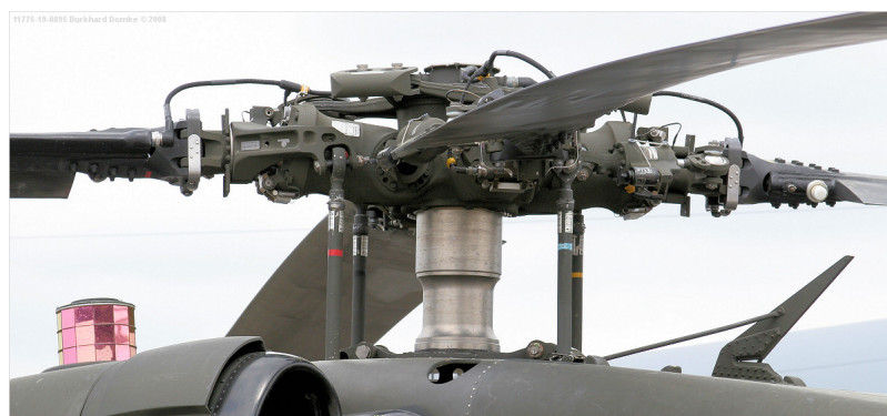
Figure 1.2. UH-60 swashplate assembly [5].
