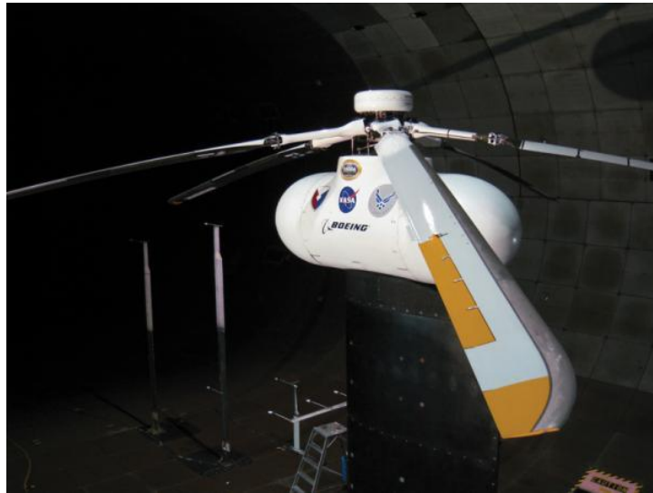
Figure 1.3. Trailing edge flap on SMART rotor [6].
